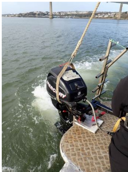
Figure 5.2 Skalmey stern platform and fixing for outboard engine
