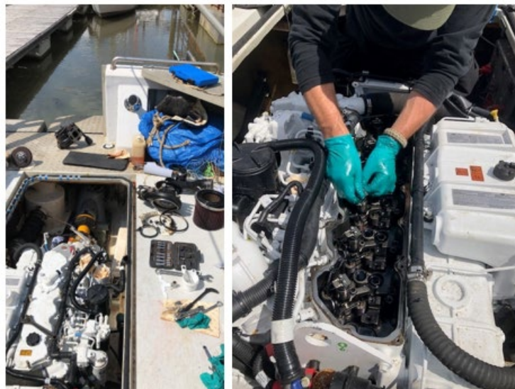
Figure 5.1 Skalmey engine repairs July 2023
