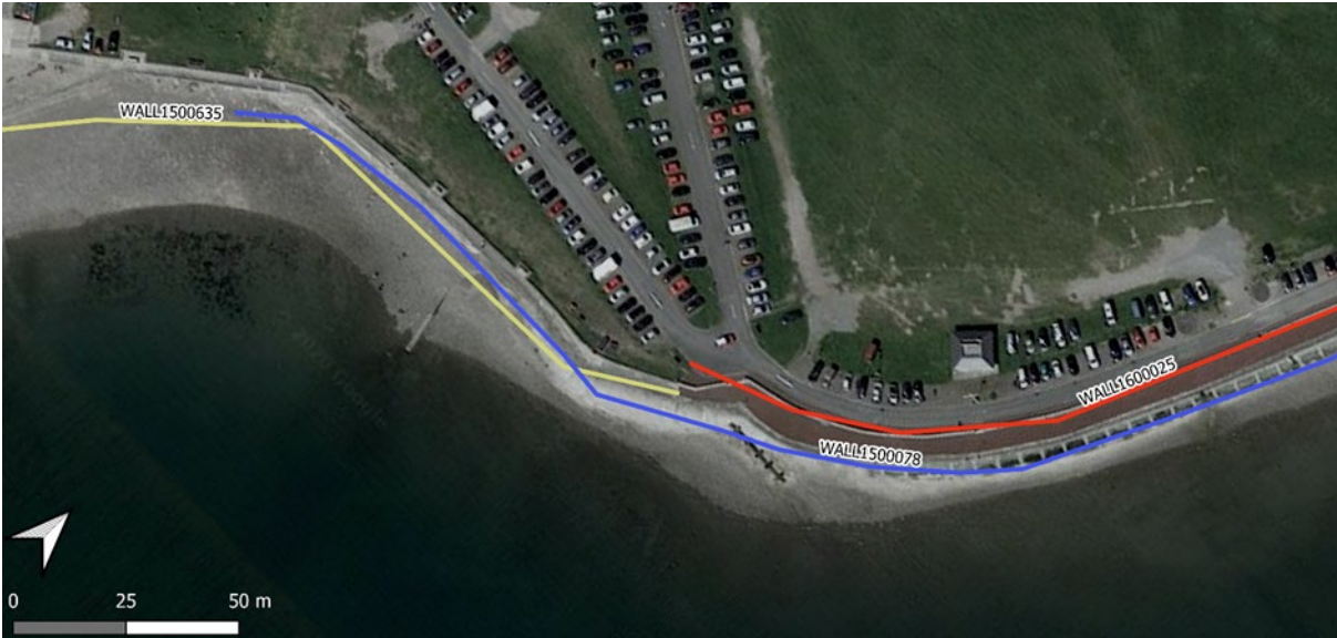
Figure 3: Planar view showing defences where there appears to be significant overlap where in reality there is only one defence
