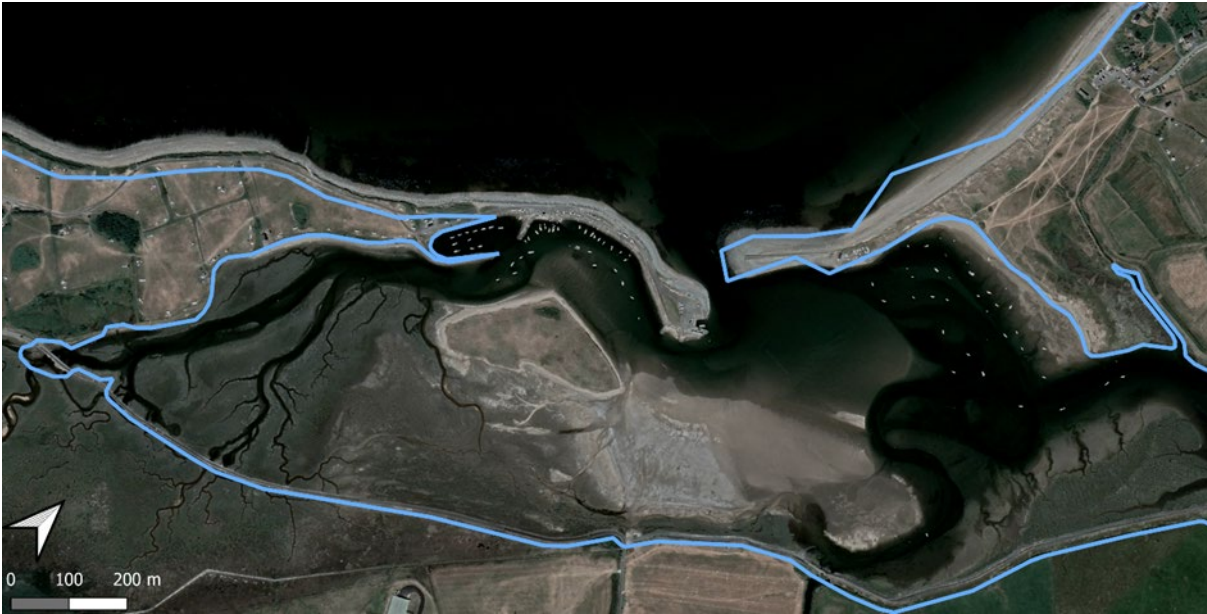
Figure 2: Inaccuracies of the shoreline management plan data (blue).
