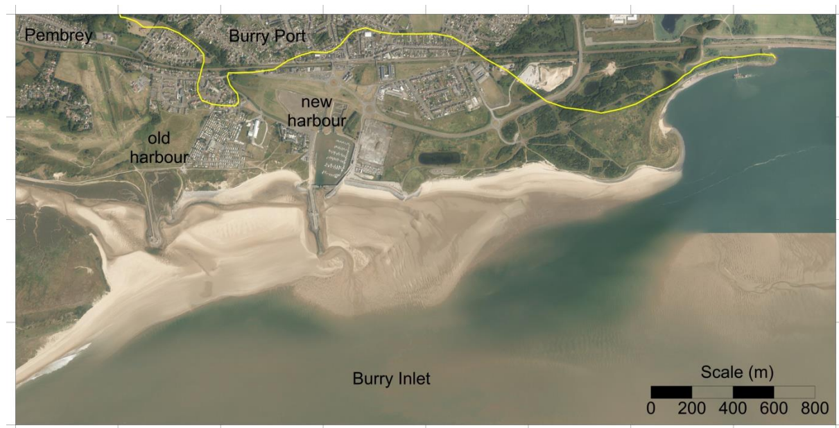
2013-14 aerial photography. The yellow line indicates the limit of blown sand based on BGS 1: 50 000 scale geological maps.
