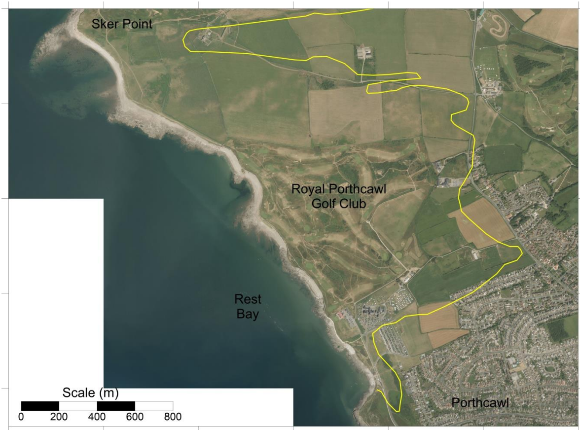
2013-14 aerial photography, flown 2013-14. The yellow line indicates the limit of blown sand based on BGS 1: 50 000 scale geological maps.
