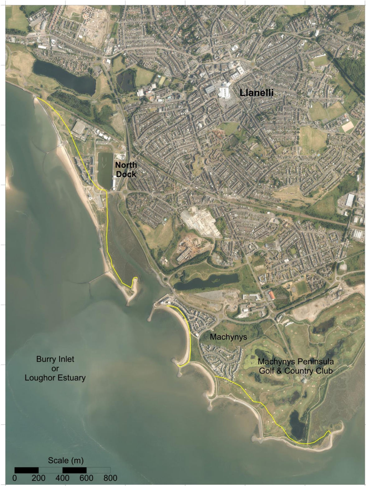
2006 and 2013-14 composite aerial photography. The yellow line indicates the limit of blown sand based on BGS 1: 50 000 scale geological maps.
