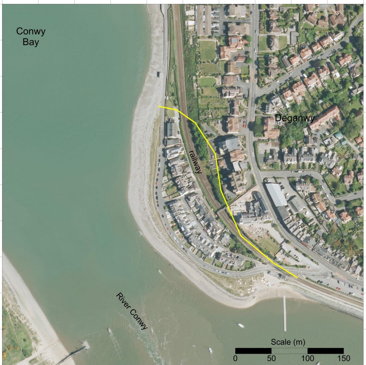
2013-14 aerial photography. The yellow line indicates the limit of blown sand based on BGS 1: 50 000 scale geological maps.
