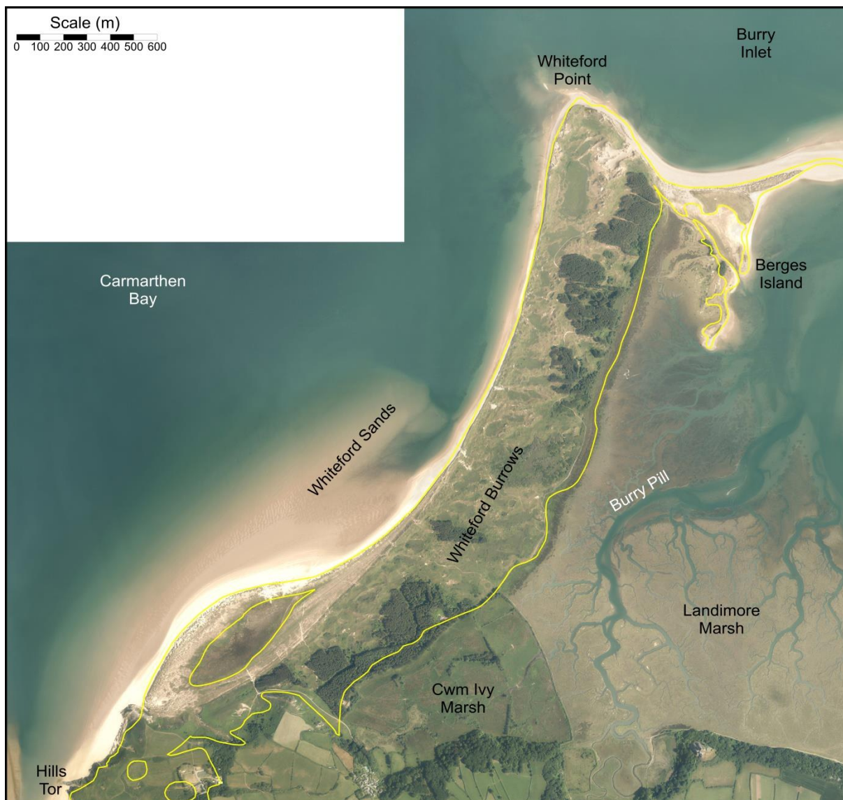
2013-14 aerial photography. The yellow line indicates the limit of blown sand based on BGS 1: 50 000 scale geological maps and KPAL ground surveys.
