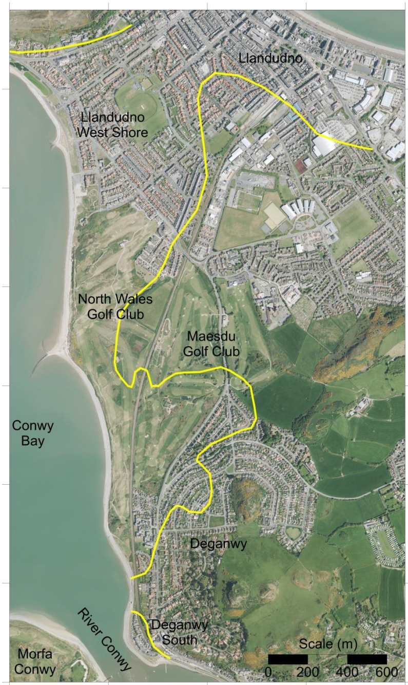
2013-14 aerial photography. The yellow line indicates the limit of blown sand based on BGS 1: 50 000 scale maps.
