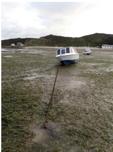
Figure 8 Mooring that consists mainly of rope (20160919 BW Porth Dinllaen 0041)
