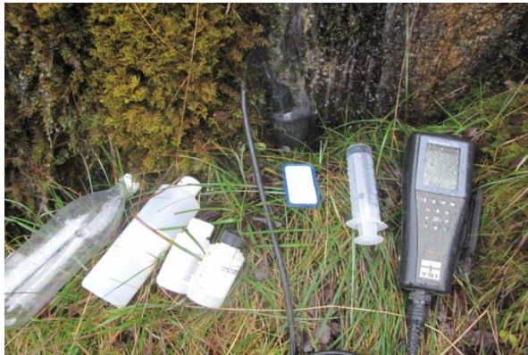
Collection of a water quality sample and field readings from seepage at the top of the site
