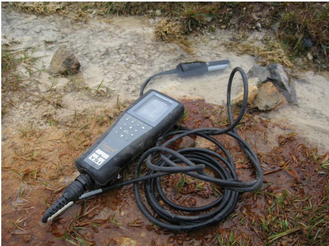
Figure 3 YSI Professional Series Fieldmeter in situ until the readings have stabilised. Foel Fawr Site 2 FF2.13 NGR SN7344419167.
