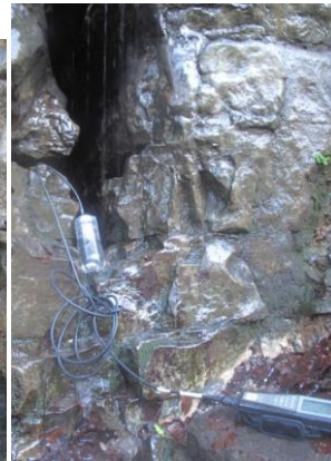
Dripping water from the cliff face collected in a container for in situ water quality testing
