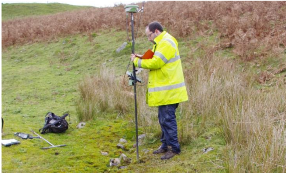
Figure 2 Surveying using the Leica Smart Rover (Blaen Onnen nr SN157170)
