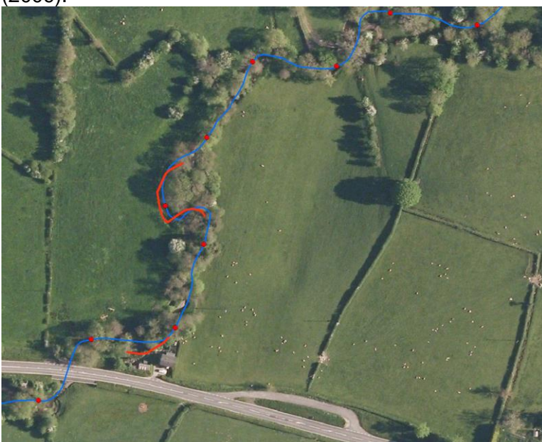
Figure 4. A small section of the Mithil Brook with aerial photography, 50m 'spot-check' markers (red circles) and the Fluvial Audit bank protection layer (red lines). Aerial imagery: Infoterrer (2009).
